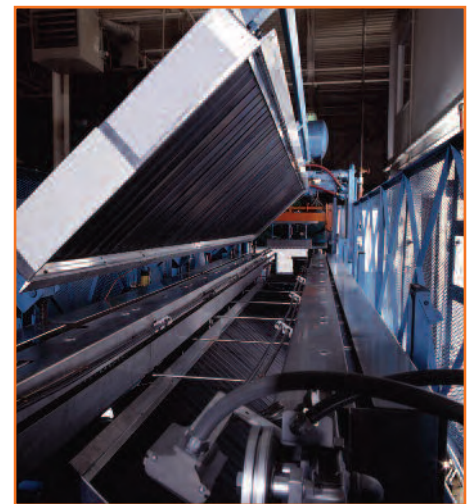
Watlow's radiant heaters allow plastic to be heated quickly and uniformly.
