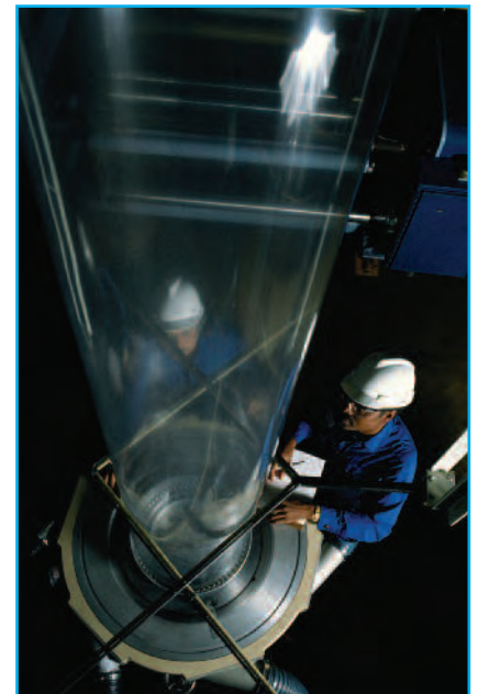
Plastic is heated in a barrel with Watlow heaters and then blown into film.
